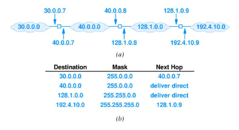
↑ Table (b) shows the routing table for the middle router in diagram (a).
